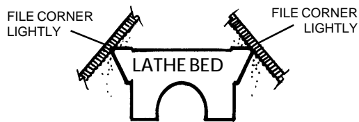
FIGURE 1—Filing corners of bed dovetail for better fit of tailstock riser block.
