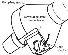
Figure 2: Adjusting shaving thickness.
